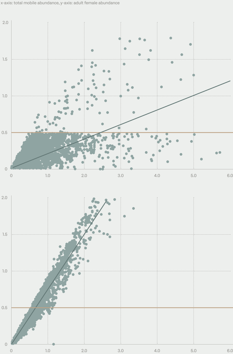
Reproduction of the "cliff effect" [129] based on manual counts from BarentsWatch data (upper panel). Stingray automated lice counts show no sign of a "cliff effect" (lower panel). Observation period: 01.01.2024 - 30.12.2024. Axis truncated at two adult females and six total mobiles.
